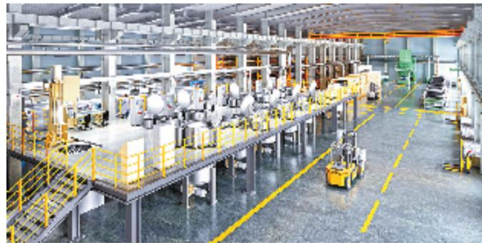
绿宇年产5000吨散棉/棉筒纱非水介质染色生产线
